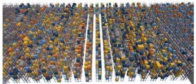
Fig. 2. Five chosen high runners spread in "chaotic" warehouse - colors mean same part number - pallet positions taken from real current WMS. The task = find some clusters.
